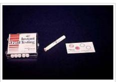
Testing kits are commercially available for detecting lead. These swabs, when wiped on a surface, turn pink in the presence of lead. but cheaper methods include running water in the morning to flush out the most contaminated water, or adjusting the water's chemistry to prevent corrosion of pipes.<sup>[111]</sup> Lead testing kits are commercially available for detecting the presence of lead in the household.<sup>[50]</sup>
