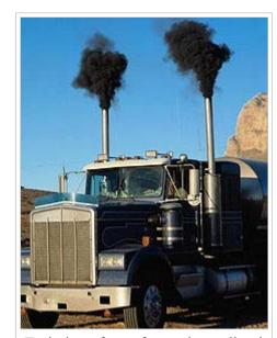
Emission of soot from a large diesel truck, without particle filters.
